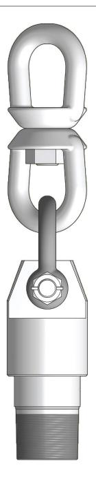
The Black Gator® Swivel Lift Nubbin allows handling of flush joint casing and tubing in an Electric Submersible Pump (ESP) bypass system. It has a pin thread to mate with the corresponding thread on the casing or tubing. A 4.75-ton swivel allows single joints to be lifted with the tugger line or crane, without the need for single joint elevators.
